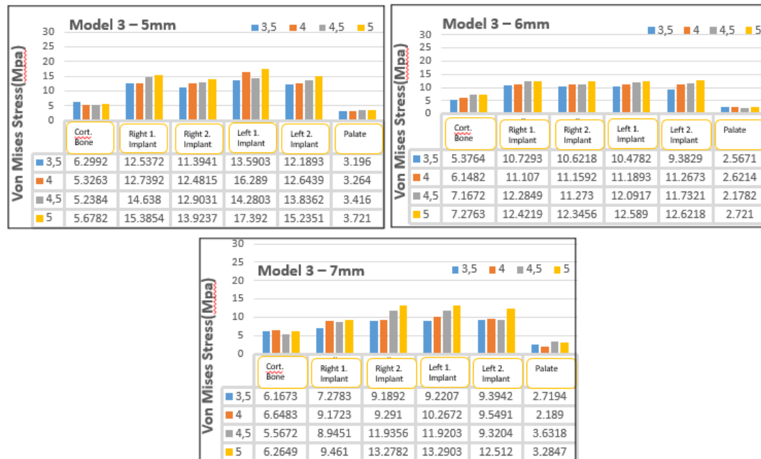
Figure 6. Results of analysis for model-3 according to implant lengths (5 mm, 6 mm and 7 mm), abutment lengths (3,5 mm, 4 mm, 4,5 mm, 5 mm) Cortical bone, palate and short dental implants (right-1. implant, right-2. Implant, left 1. implant, left 2. implant)
