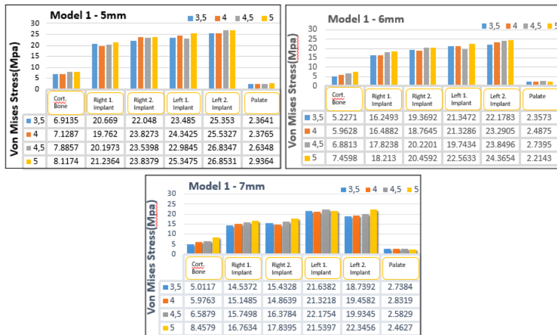
Figure 4. Results of analysis for model-1 according to implant lengths (5 mm, 6 mm and 7 mm), abutment lengths (3,5 mm, 4 mm, 4,5 mm, 5 mm) Cortical bone, palate and short dental implants (right-1. implant, right-2. Implant, left 1. implant, left 2. implant)
