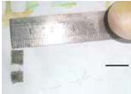
Figure 2: The nitinol wires 0.125 mm in diameter and 5 mm long, scale bar: 10 mm
